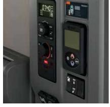
**Convenient controls.** Adjust sleeper heating/cooling and the audio system from the sleeper control panel. Need to be noticed? Just press the "panic" button to call attention to your vehicle. The control panel in the VNL 740, 760, and 860 sleepers includes controls for lighting, locks, and the inverter, as well as charging and audio ports.
