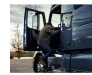
Easy in and out. Doors are 3+ feet wide, 4+ feet high, and open a full 70 degrees for ease of access. Ergonomically-placed, internal grab handles prove the safest and most secure way in and way out of the cab.
