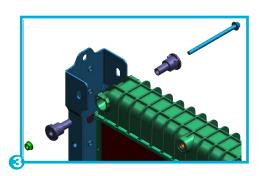
New through tank isolator design allows for maximum thermal cycle and vibration life.
