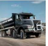
The Power Launch feature is a part of the performance software package. It is activated to provide extra torque when starting from a standstill, when loaded to capacity, or on poor terrain. The feature matches torgue to the terrain, minimizing wheel-slip on soft surfaces.
