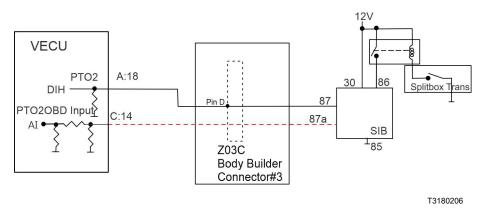
**Note:** Body builder will add the wire from the VECU pin C:14 to the body builder connection.
