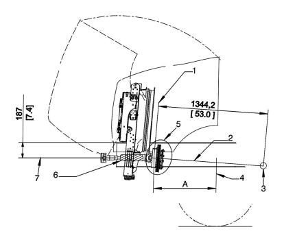
Fig. 2 Front PTO, Axle Back, With 1240 Sq. in. Radiator
