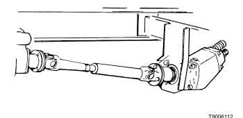
The same requirements apply to power take-off propeller shafts as for drive line propeller shafts. For best service life, the true joint angle should be kept between 0.5 - 8 degrees.
