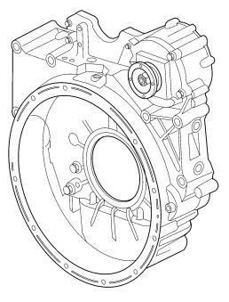
Rear-Mounted Engine PTO (D13 engine)
