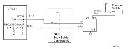
Note: Body builder will add the wire from the VECU pin C:14 to the body builder connection.
