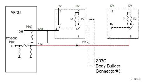
Note: Body builder will add the wire from the VECU pin C:14 to the body builder connection.
