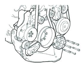
Fig. 5 Crankshaft Vibration Damper
